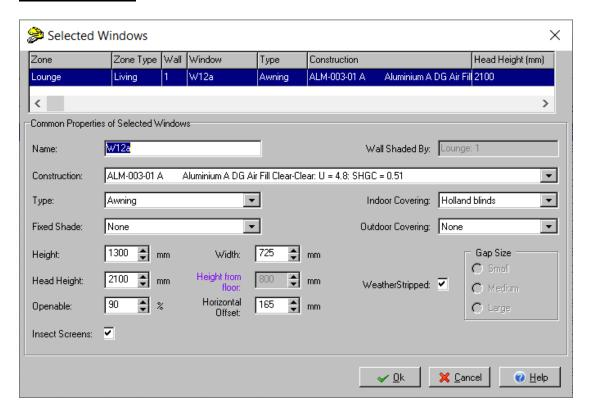
For windows, infiltration inputs are only allowed to modify for existing building and renovation, not allowed for new building in rating mode.
